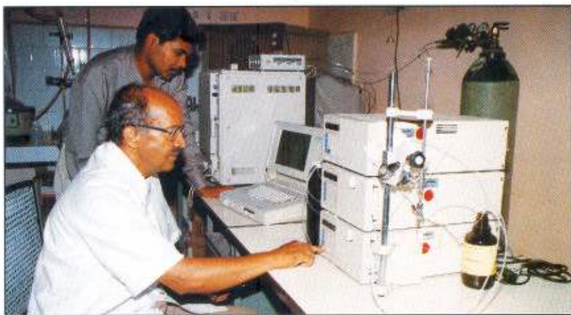
High performance liquid chromatograph for analytical work
